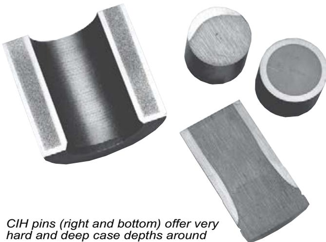
*CIH pins (right and bottom) offer very hard and deep case depths around the full circumference of the pin. SIH pins (upper left) are hardened only on the load bearing surface so shock can be better absorbed by the back of the pin.*
